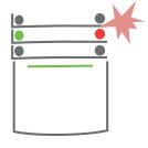
3. Unsetting is finished and sirens are silenced. The green flashing button indicates unsetting of the particular section. The red flashing light indicates alarm memory.
